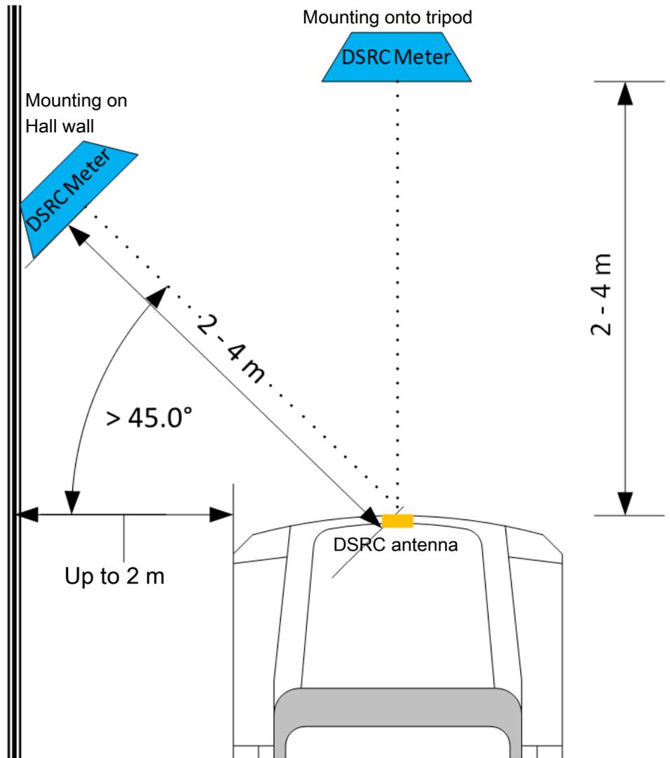
Fig. 11: Permanent installation or mobile use of the DSRC meter
