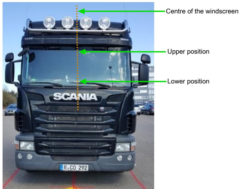
Fig. 2: Possible installation locations of the DSRC antenna
