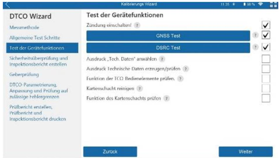
After a successful GNSS- and DSRC test, the inspection is continued as usual.
