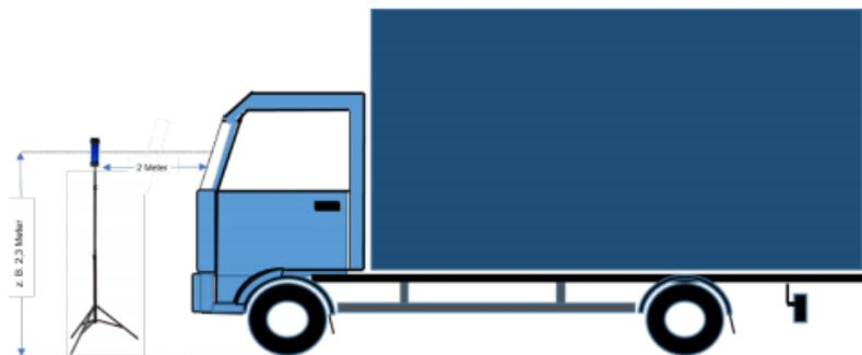
Fig. 10: Use of the DSRC meter in the workshop
