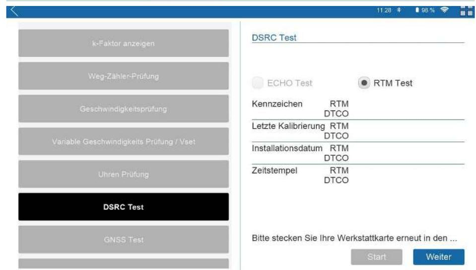
⇒ The **Start** interface is not active as the workshop card is not yet inserted into the WorkshopTab.
