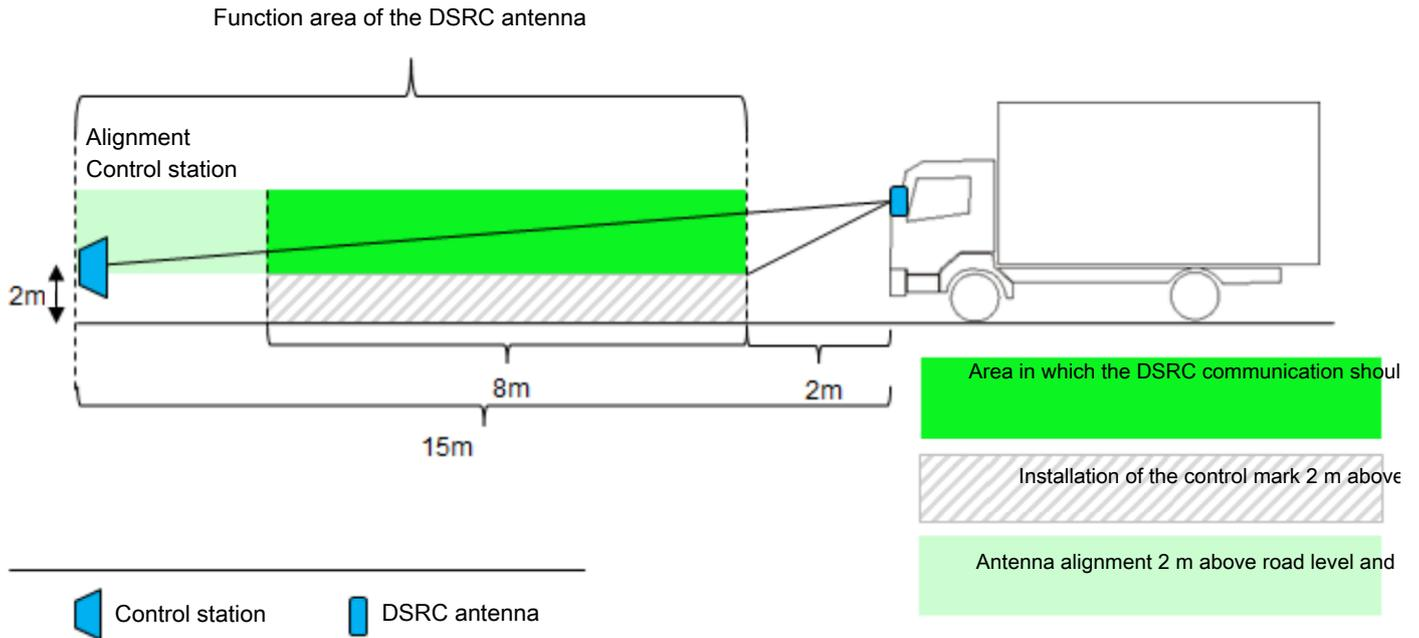
Fig. 1: Function area of the DSRC antenna
