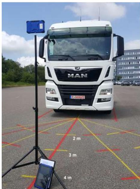
Fig. 4: Echo measurement using a tripod
